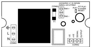
The terminal block CONN3 is provided for the connection of an optional NC941B remote battery back-up kit. <u>Do not</u> <u>connect any other type of battery back-up facility to this</u> <u>unit.</u> (See NC941B installation instructions for battery connection details).
